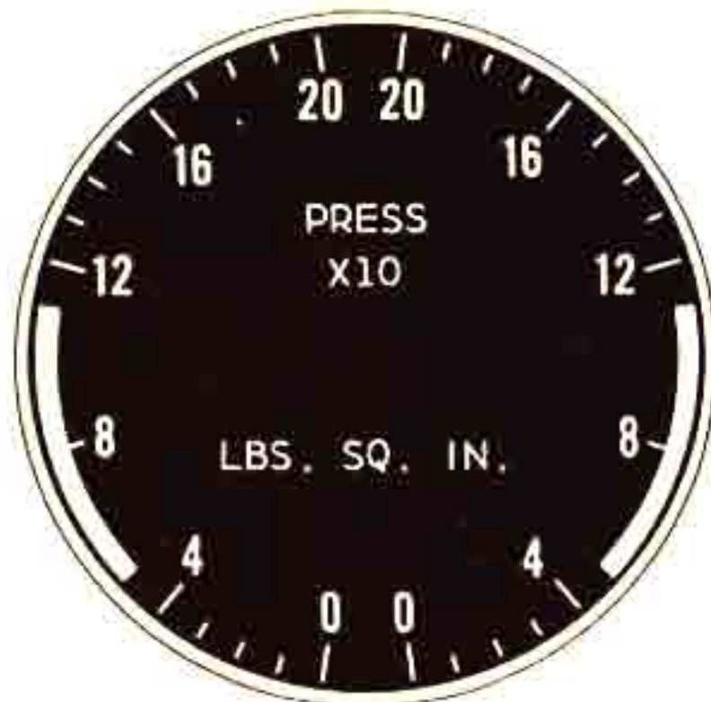
OIL PRESSURE 50 To 110 PSI Operating Range
