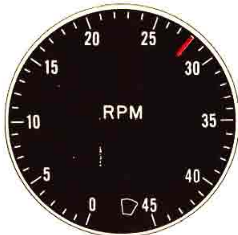
TACHOMETER 2800 RPM Maximum Take-off and Military Power
